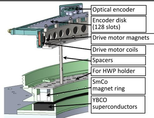
• We employ a custom AC driver motor which outputs a 3-phase signal to accelerate and maintain the rotor/HWP at a constant rotational frequency.
