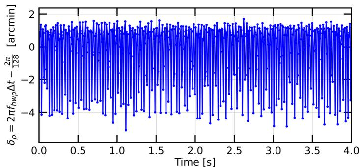
• HWP angle reconstruction is critical for data analysis. We evaluate the instability in the HWP angle using the period of the encoder.
